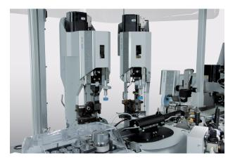
▲ Alpha 356 With crimping module and seal loading module
