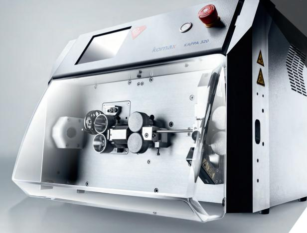
Cutting force, high volume output and advanced sensor technology make the Kappa machines the number one choice for automated cutting and stripping, even for smaller wire cross-sections. The machines can be used very efficiently thanks to their simple, intuitive control elements.
