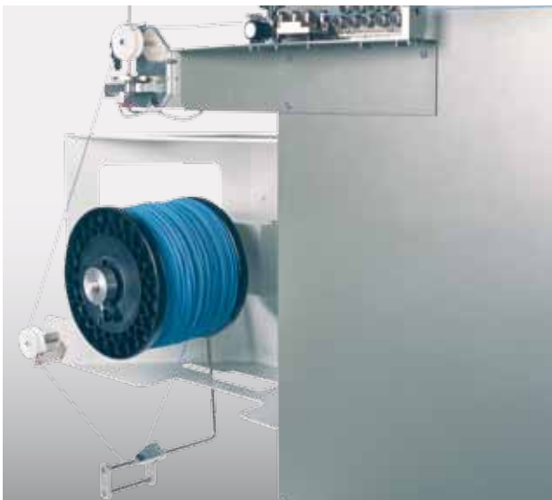
▲ Komax 104 passive de-reeler on Gamma 255
